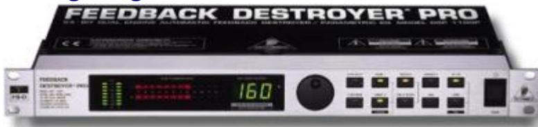
In the DSP1124P default configuration Midi comms are disabled. To enable the Midi features used by REW, the unit's Midi menus need to be set up as follows (all buttons referred to are on the DSP1124P front panel):
