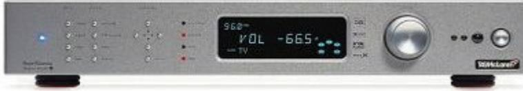
AV32R Dual Processor and AV192R support serial communication via a TAGtronic Programming Cable. The serial format is 115.2kBaud, 8 data bits, no parity, 1 stop bit. The Programming Cable converts RS232 levels to the RS485 levels of the TAGtronic bus. Only connect the black plug (to the "out" socket) for communication with REW.
